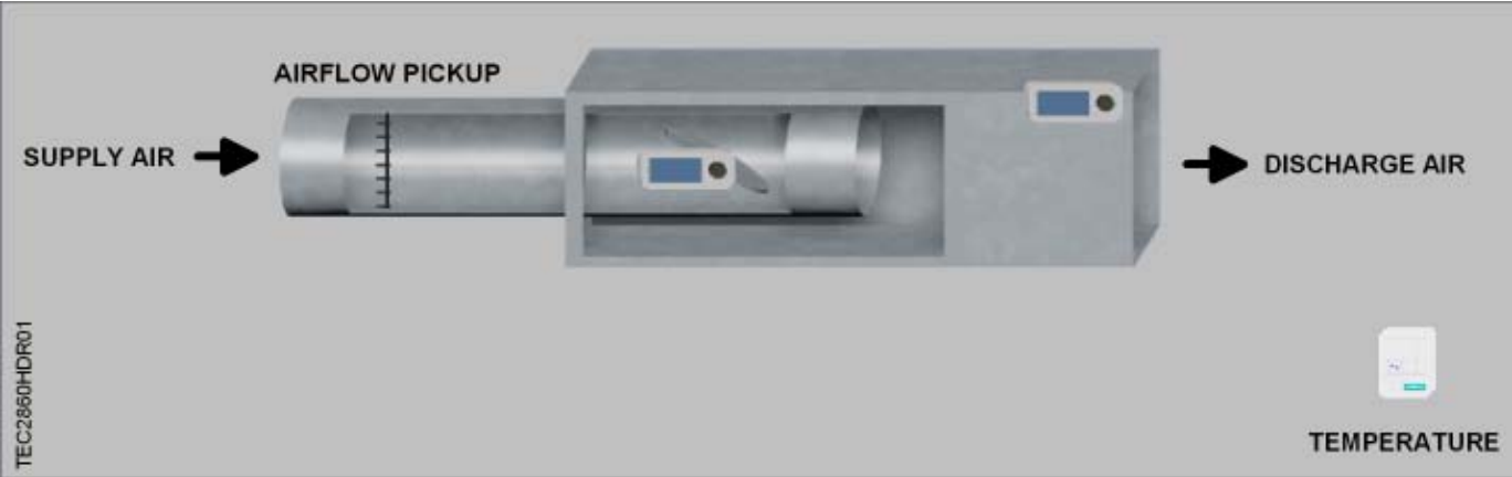
Application 2860 Cooling Only Hardware Diagram.
